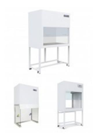
Vertical Laminar Flow Cabinets LVC-3000 Series is a work bench or similar enclosure, which creates a particle-free working environment by taking air through a filtration system and exhausting it across a work surface in a laminar or unidirectional air stream. The laminar flow cabinet is enclosed on the sides and kept under constant positive pressure in order to prevent the infiltration of contaminated room air.
