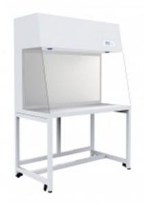
Horizontal Laminar Flow Cabinet LHC-1000 Series is a work bench, which creates a particle-free working environment by taking air through a filtration system and exhausting it across a work surface in a laminar or unidirectional air stream. The laminar flow cabinet is enclosed on the sides and kept under constant positive pressure in order to prevent the infiltration of contaminated room air.
