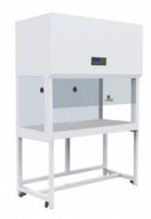
Vertical Laminar Flow Cabinets LVC-2000 Series is a work bench or similar enclosure, which creates a particle-free working environment by taking air through a filtration system and exhausting it across a work surface in a laminar or unidirectional air stream. The laminar flow cabinet is enclosed on the sides and kept under constant positive pressure in order to prevent the infiltration of contaminated room air.
