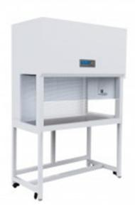
Horizontal Laminar Flow Cabinets LHC-2000 Series offers particle-free working environment by taking air through a filtration system and exhausting it across a work surface in a laminar or unidirectional air stream. The laminar flow cabinet is enclosed on the sides and kept under constant positive pressure in order to prevent the infiltration of contaminated room air.
